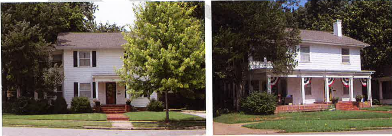
B.5.1 On the left is a house before a porch was added. On the right is an example of an addition to an existing porch. This addition maintains the character by recessing the new additions on either side of the original porch while matching the scale, rhythm and detailing of the original porch.
